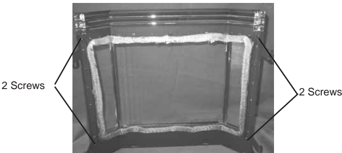
Figure 8.1 Remove the door from the appliance. Remove the existing black crown by removing the four screws on the back side of the face, and pull the crown off the door.
